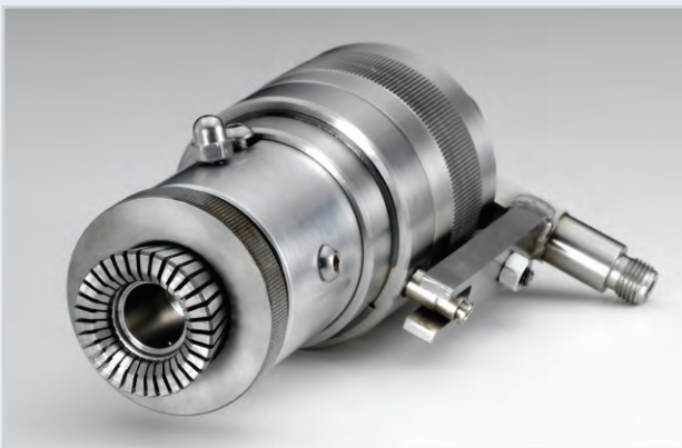
Below: crimping head for 20 mm valves. Bottom right: close-up of the crimping jaw. The 32 petals enable precision of 0.05 mm in crimping. The crimping jaw is manufactured with a special material that enables 3 million maintenance-free cycles. Bottom left: same crimping jaw with container and 20 mm mounting cup.
