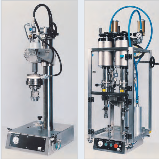
Above: left, semi-automatic unit for crimping; right, semi-automatic unit for propellant filling. Semiautomatic units are suitable for laboratory and/or small-scale production (20-25 CPM).
