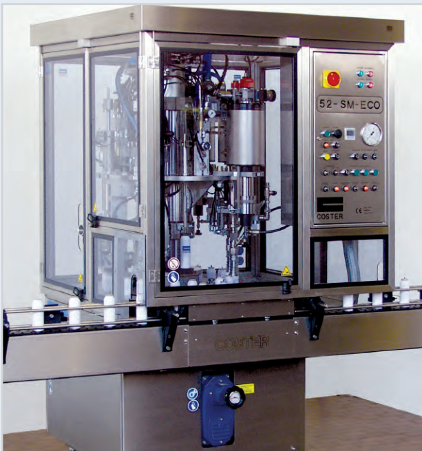
Above: automatic indexing unit for filling pharmaceutical products either in standard aerosol or dual-compartment systems (Bag-On-Valve). Line speed up to 60 CPM.
